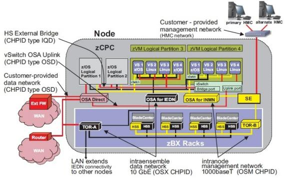
Networks in an ensemble with an vSwitch Uplink to a customer-provided data network
