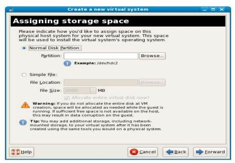
Figure 6: Storage Allocation for Virtual Machines in the Physical System
