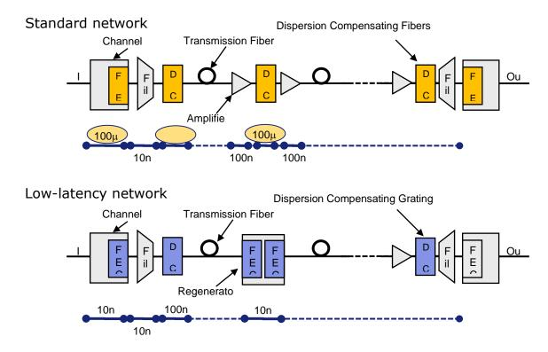
Figure 1 – Typical latency reductions achievable in long distance, ultra low latency networks (after ref. [5]).
